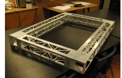
Skunkworks base frame ready to be welded together
